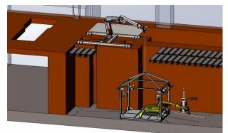
Designs for a remotely controlled equipment to remove SNF from Building No 5 in Andreeva Bay
